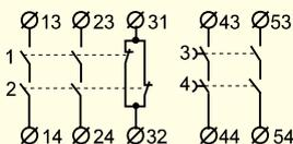
The RT7 has four (4 NO) safety outputs of which two can be delayed, and 1 NC information output.
