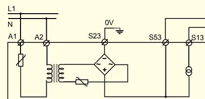
The RT7 AC option should be supplied with the appropriate supply voltage via connections A1 and A2.
