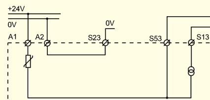
The RT7 DC option should be supplied with +24 V on A1 and 0 V on A2.
