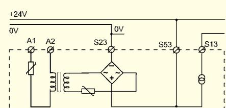
All AC-units can also be supplied by +24 VDC to S53 (0VDC to S23).
