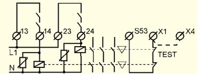
Contactors, relays and valves can be supervised by connecting 'test' contacts between S53 and X1. Both manual supervised and automatic reset can be used.
